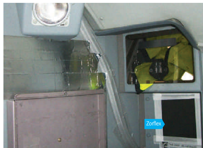
Zorflex pure fabric placed in the cabin area to adsorb 'interfering' molecules.
